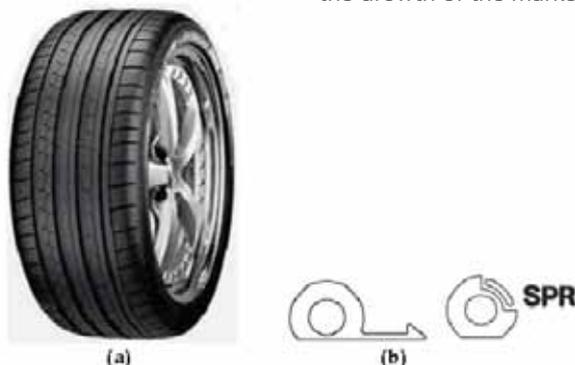
Fig.5: Typical Run Flat Tyres
